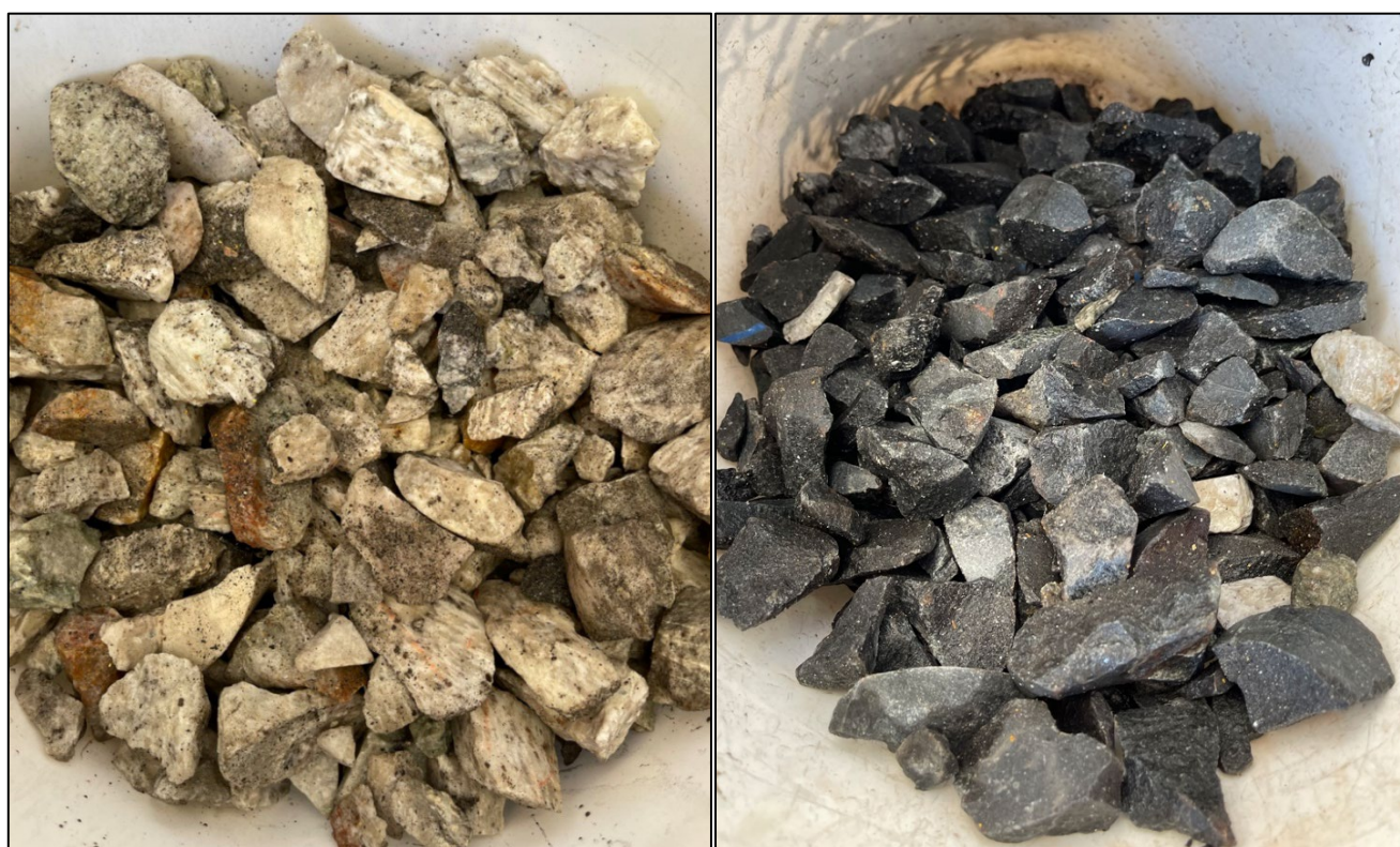
Figure 3. Ore sorter product streams, Accepts (Left) and Rejects (Right)
