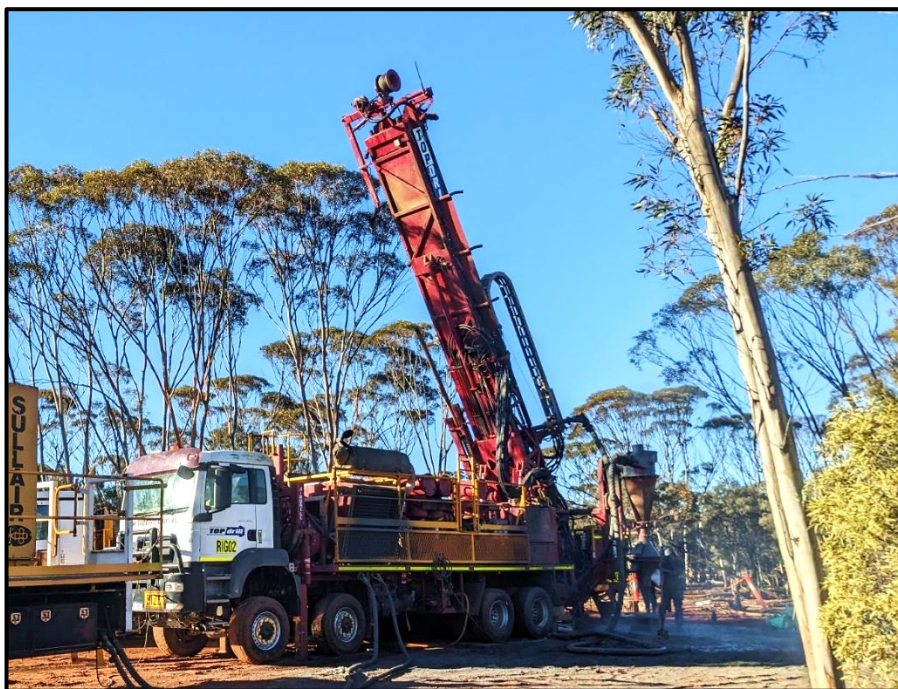
Figure 1 – RC Drilling underway at Galileo's Norseman Project
