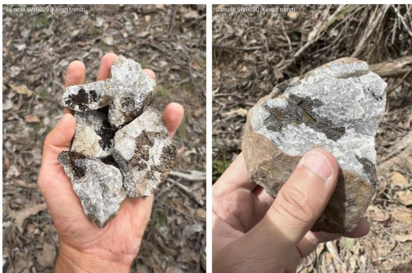
Figure 8. Large cassiterite (tin-oxide) dark mineral crystals and aggregates, from the Sweetwater area: L) Sample SWR029 (16.70% \text{SnO}_2 ) and R) Sample SWR030 (8.65% \text{SnO}_2 )
