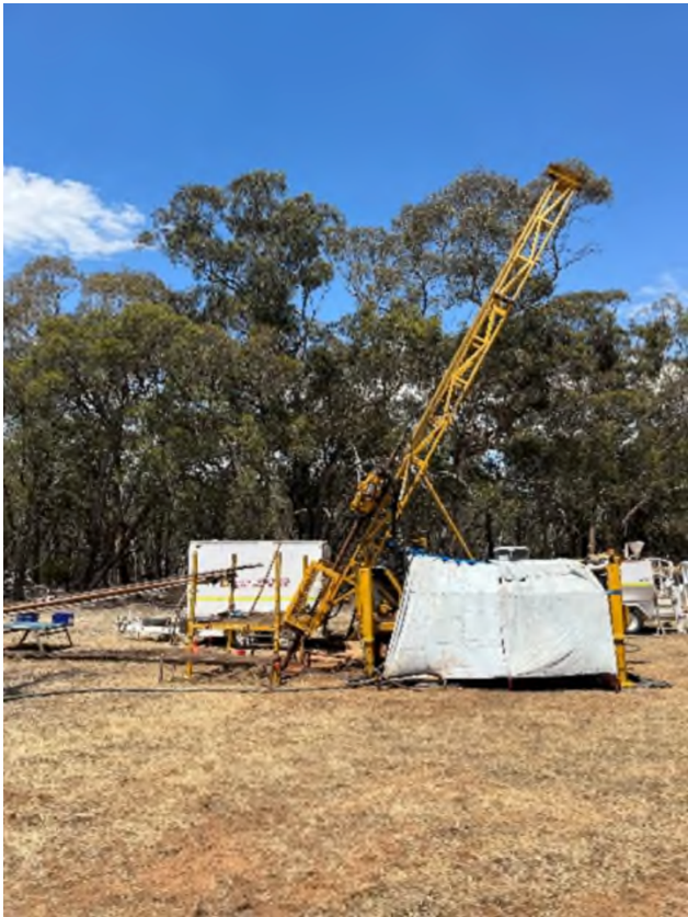
Figure 2 - Irvine Project (Stawell zone) – Diamond drill rig in operation with covering noise attenuation materials
