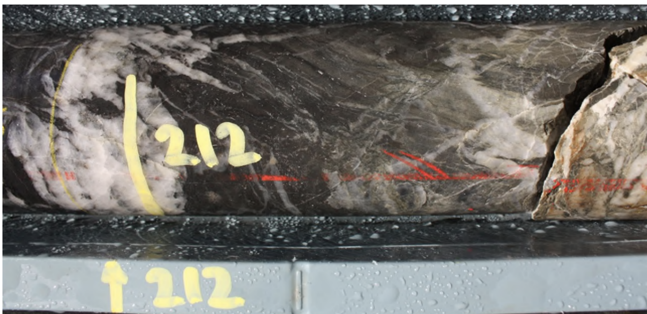
Figure 6 - RD045. 212.00 212.20m Acicular arsenopyrite needles developed adjacent to steeply inclined shear structure within overlying western sediments 9
