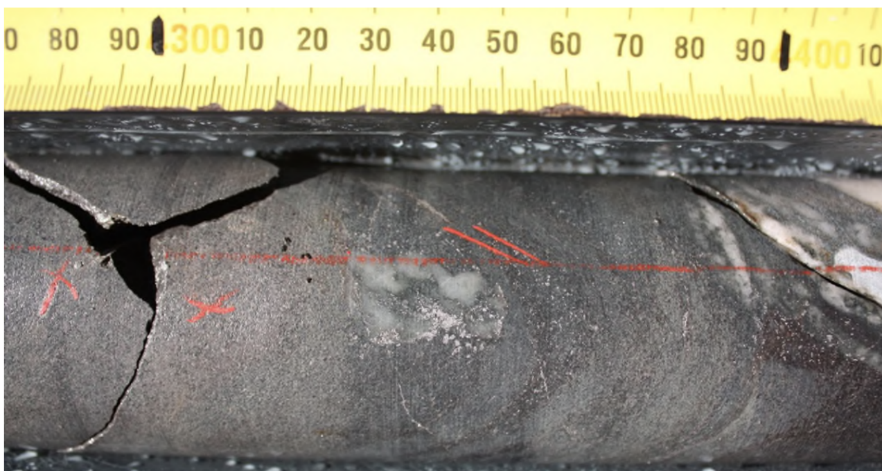
Figure 8 - RD045 406.2 – 406.3. fine grained arsenopyrite intergrowth around silica within disseminated pyrrhotite groundmass.
