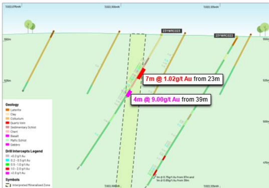
Figure 2: Cross section at Barwidgee Fault Prospect drilling.
