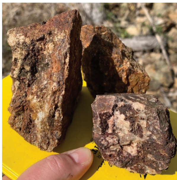
Figure 2. Rock Chip sample MRRK072, 6.06g/t Au, 1.5% Cu, 585g/t Ag
