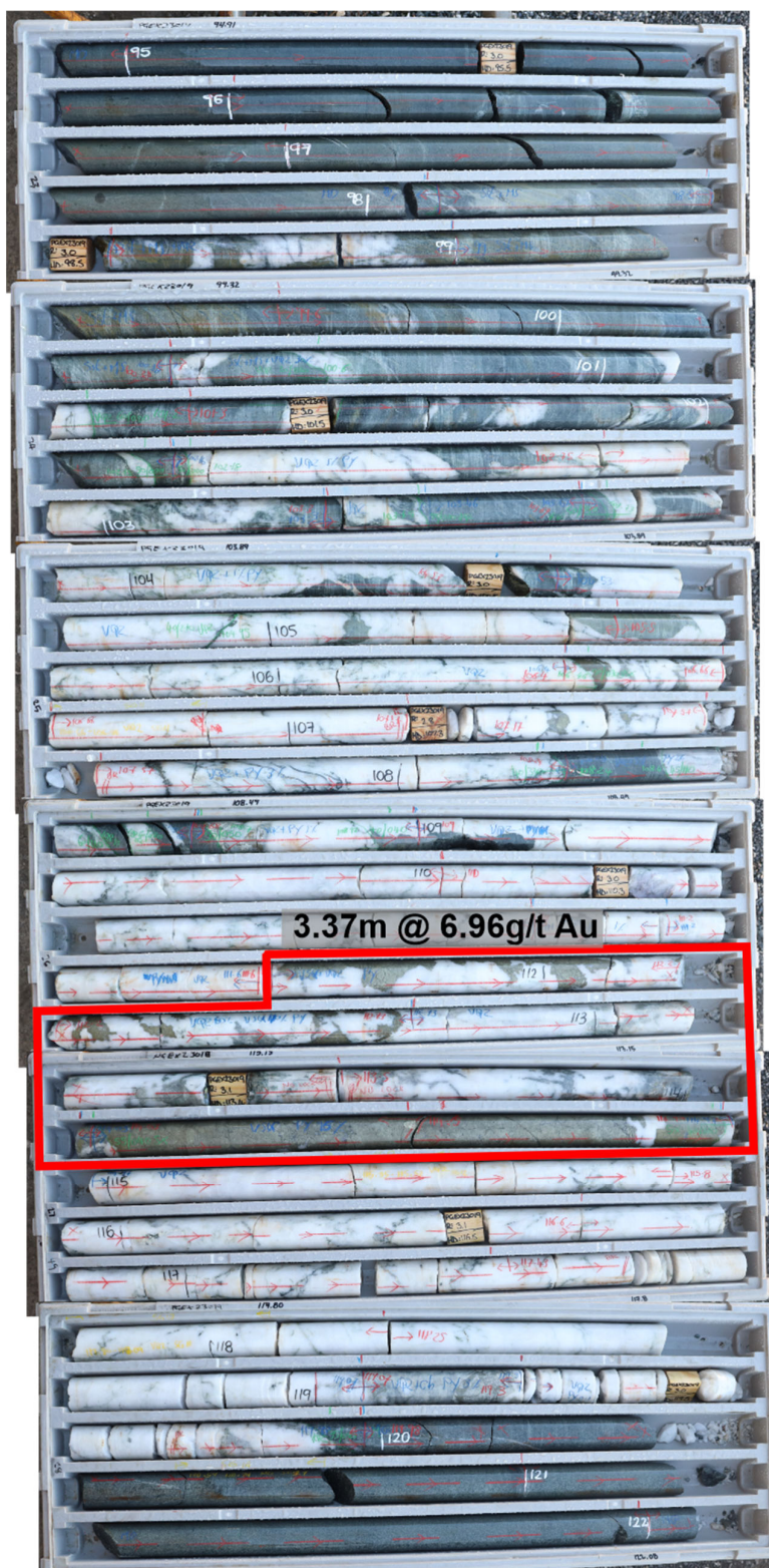
Figure 5: Core photo of PGEX23019 showing the wide zone of quartz-pyrite veining and the significant intercept of 3.37m @ 6.96 g/t Au.
