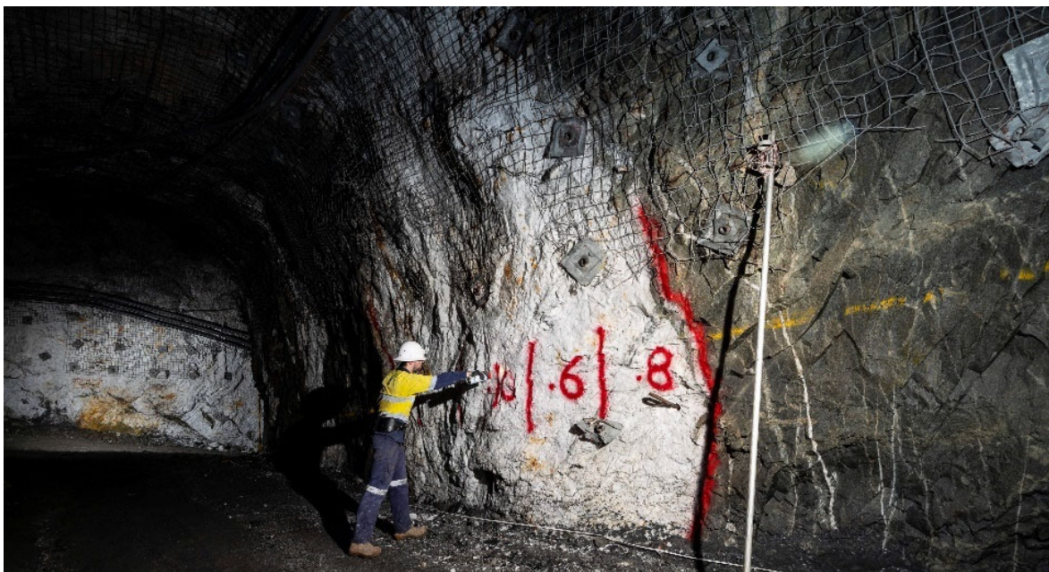
Figure 1: Quartz-pyrite lode veining in the Paulsens decline at the 154 level. This is the interpreted exposure of the thick (up to 52m wide) quartz-pyrite mineralised zone that extends the Main Zone for at least 175m.
