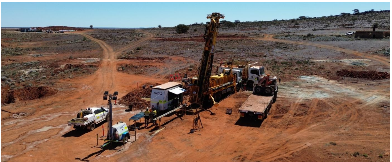
Figure 2: Diamond drill rig in action at the Island Gold Project, October 2025
