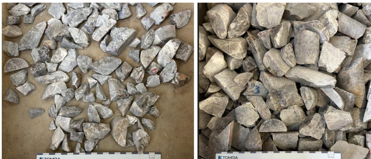
Figure 3: Left - 20.0% \text{Cs}_2\text{O} pollucite concentrate (12.5 to 25 mm fraction); Right - 11.5% \text{Cs}_2\text{O} pollucite concentrate (+25 mm fraction). See Table 1, Figure 5, and news release dated April 9, 2025 , for drill hole composite sample intervals, location, and assay data.
