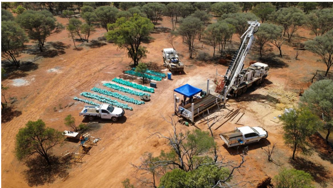
Figure 2: Resolution Drilling diamond rig on site at the Percival Prospect, North Cobar.
