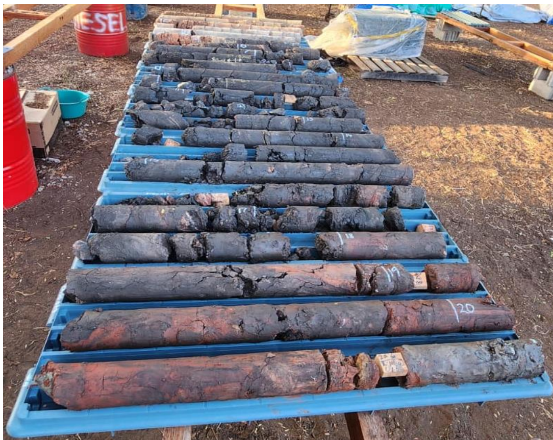
Figure 7: Secondary manganese in core from EMDD033, looking from the bottom of the hole.
