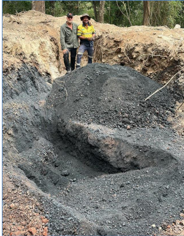
Figure 2: In-situ secondary enrichment manganese mineralisation identified during trenching 1
