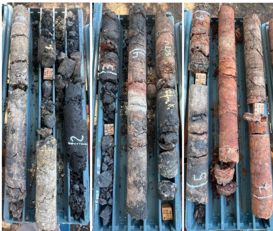
Figure 6: Secondary and detrital manganese in EMDD026.
