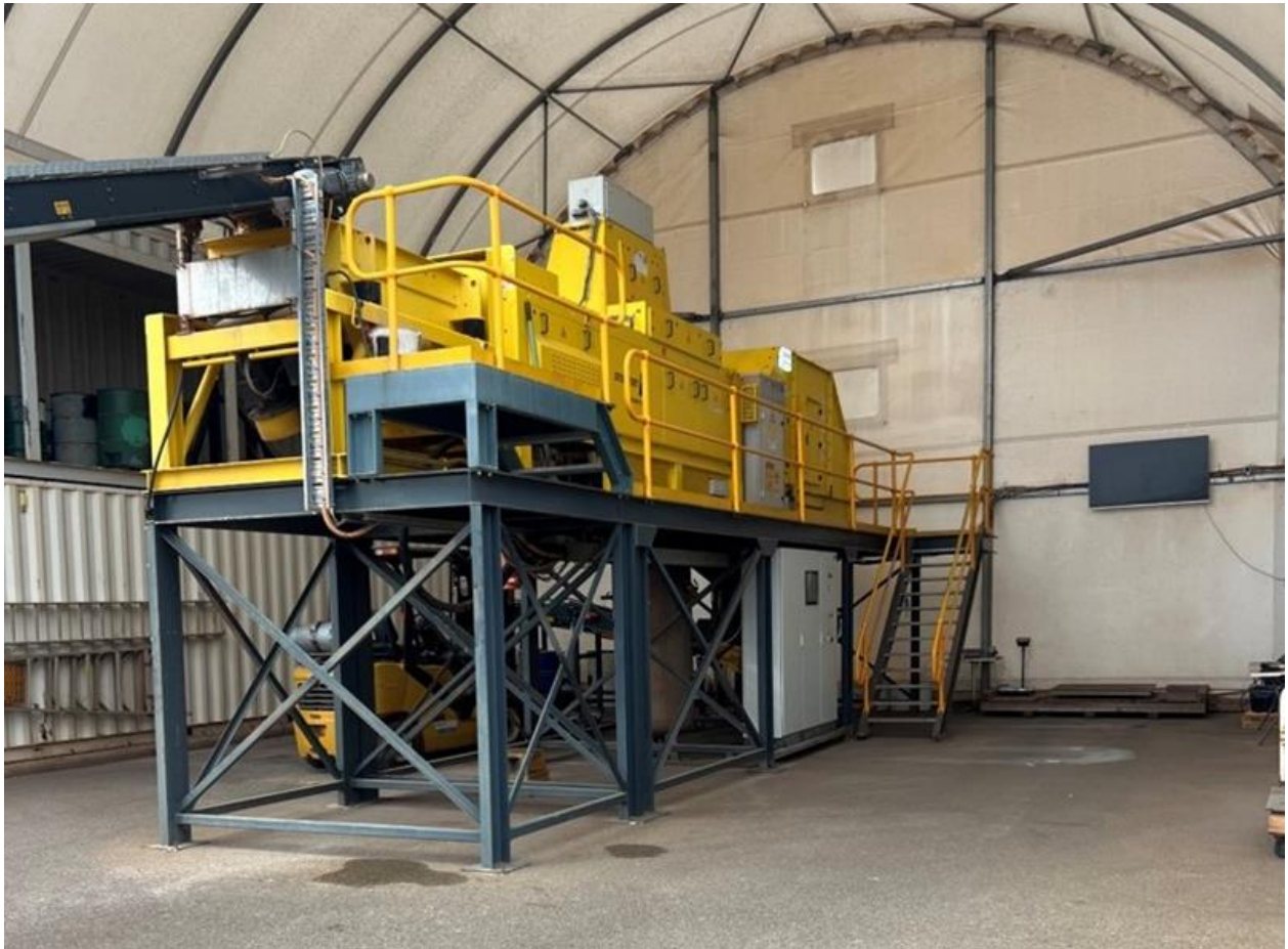
Figure 2 – Steinert Ore Sorter used in the testwork
