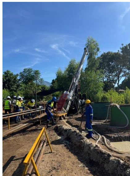
Figure 2 Diamond drill rig in operation
