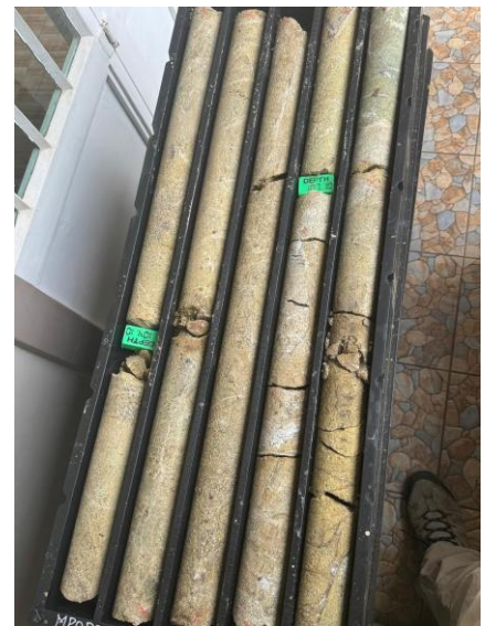
Figure 3 Diamond core trays
