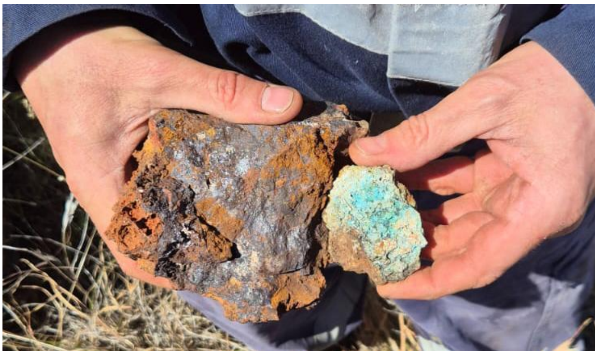
Figure 3 - Gossan outcrop (482389E, 7438704N) showing classic ex-sulphide boxwork texture identified at VT1 immediately along strike from outcropping Oonagalabi Formation marble with oxidised copper mineralisation present. Note: Visual estimates of mineral abundance results should never be considered a proxy or substitute for laboratory analyses where concentrations of grades are the factors of principal economic interest. Visual estimates also potentially provide no information regarding impurities or deleterious physical properties relevant to valuation.
