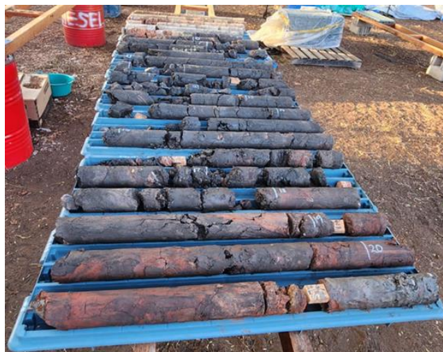
Figure 1: EMDD033 drill-core showing the 11.97m interval of mineralisation
