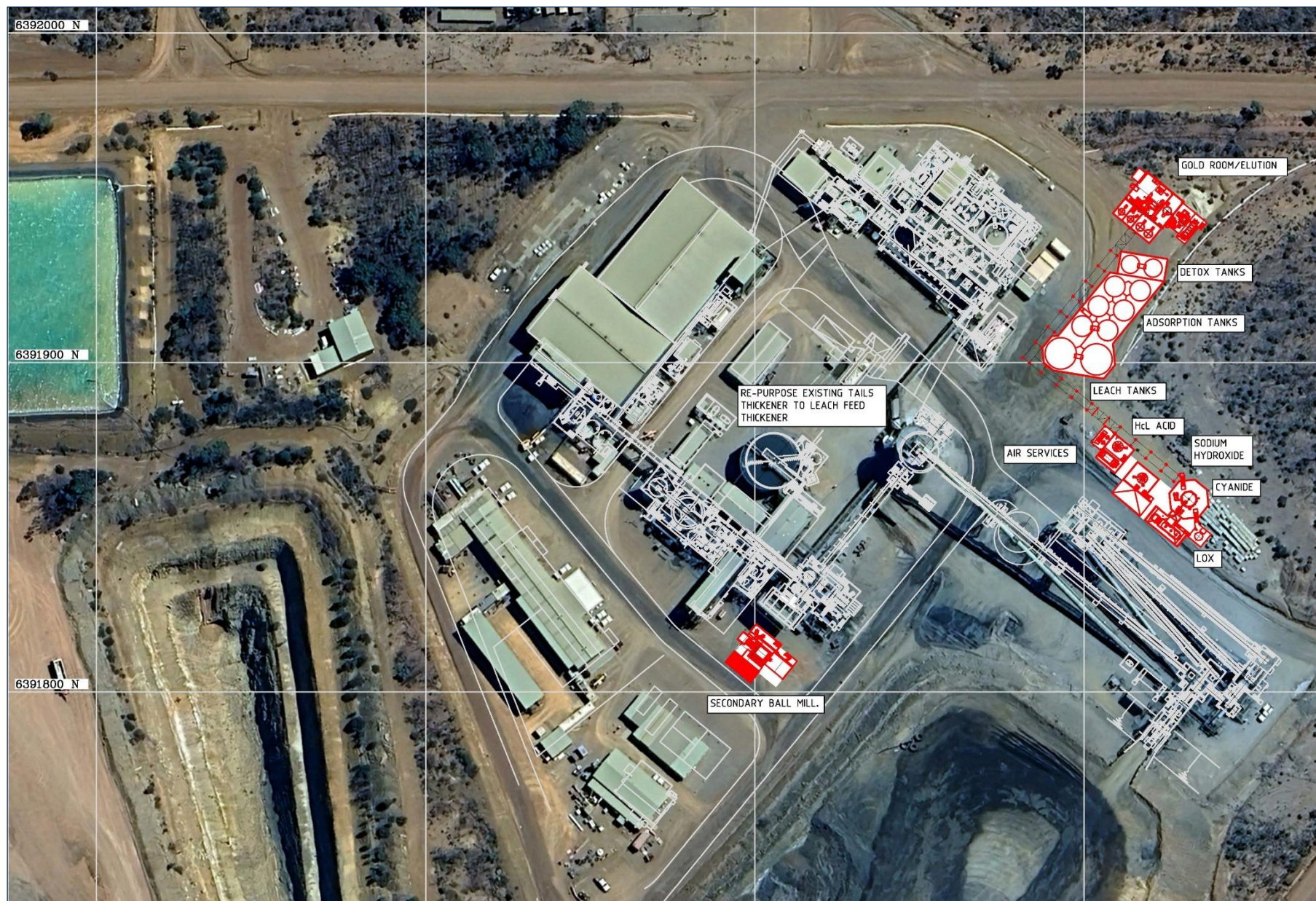
Figure 3: Cosmic Boy Concentrator with proposed modifications (red).
