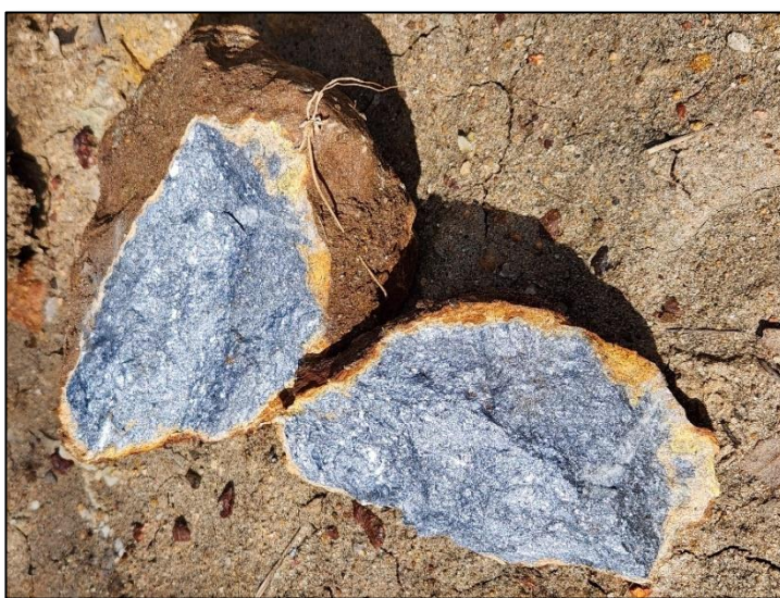
Figure 1: Massive Stibnite from sample BSE04 returning 55.5% Sb
