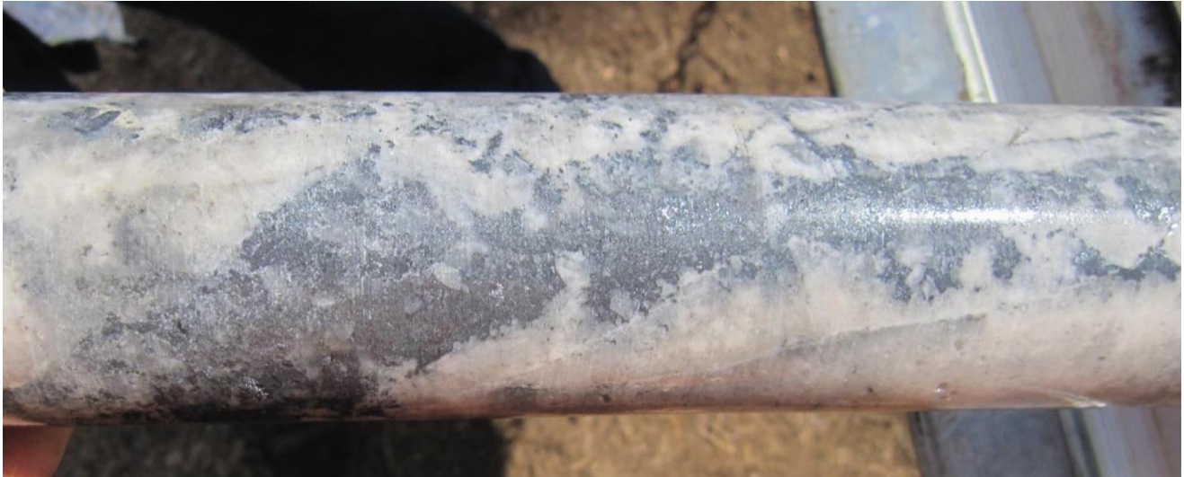
Figure 5: The Banshee core pictured, drill hole CNDD01 89.9m-90.2m, was part of a zone that assayed 1.25m @ 5.23% Sb and 1.39g/t Au (ASX: GDM Prospectus 2023 and ASX: GDM Sep 2024 ).
