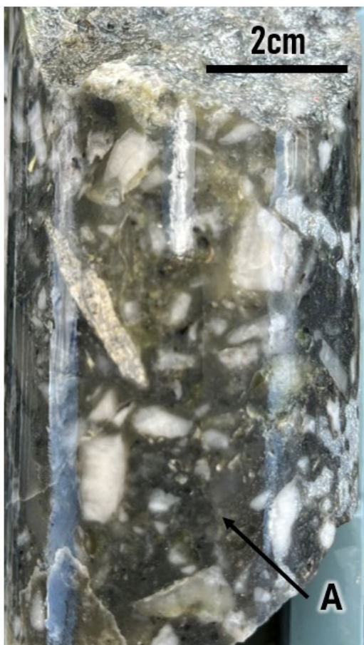
Figure 7: Hydrothermal quartz breccia with black silica sulphide matrix (A) & chalcopyrite rich clasts (~2%) (B) from A Vein in 25FCDD010.
