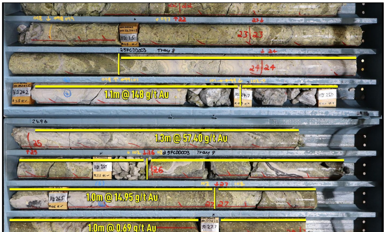
Figure 2: High-grade epithermal gold intersection from 25FCDD003. Core photography annotated with gold intersections and assays.
