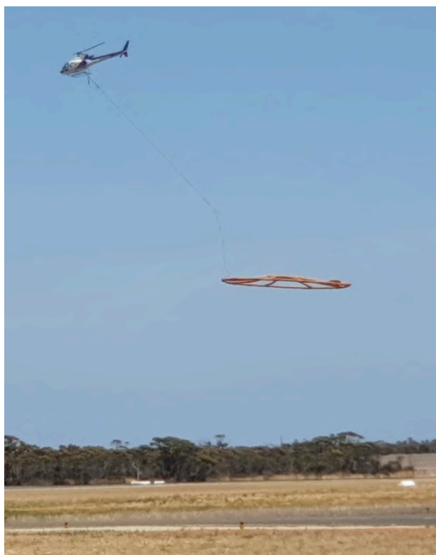
Figure 2:6 Squirrel helicopter with NRG's Xcite electromagnetic system on site
