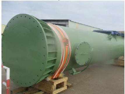
Main Venturi Scrubber
