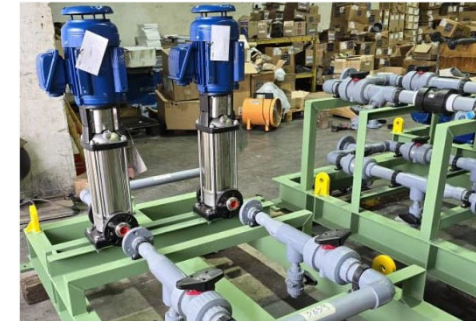
Cloth Wash Pumps Skid
