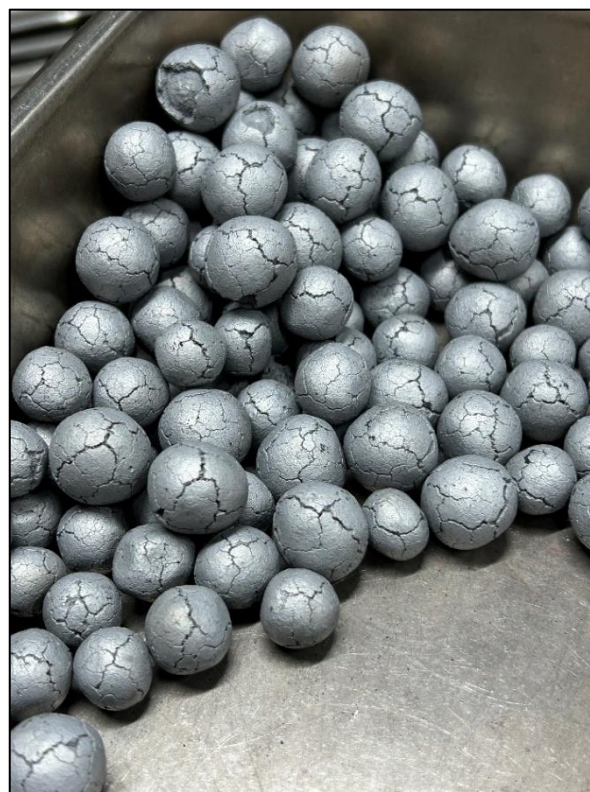
Figure 1: Pellets after Linder metallisation / reduction
