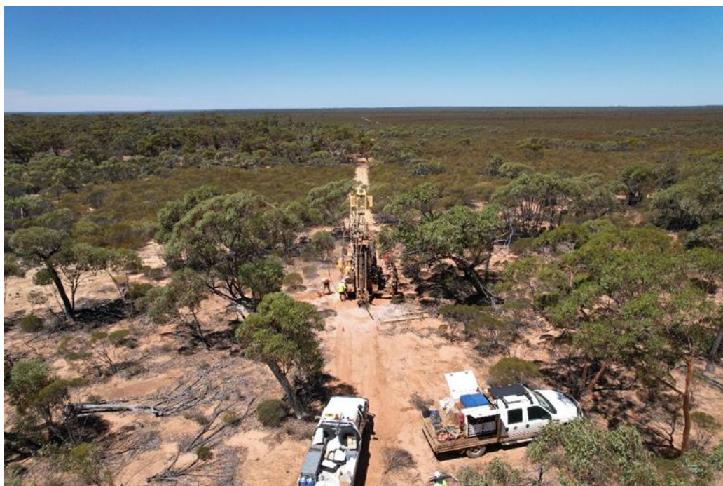
Fig. 1 - Aircore Drilling at the Claw Project - February 2025
