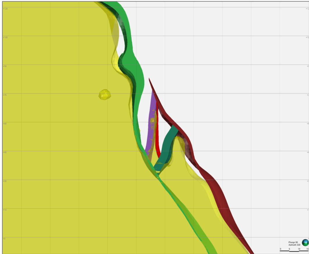
Figure 9: Trinity Domain Cross Section. West Edge domain in Green, West Waterloo East Wall domain in Purple, East Waterloo West Edge domain in red, East Waterloo East Edge in Dark Green and Lower West domain in dark red, basalt interpretation shown in yellow.
