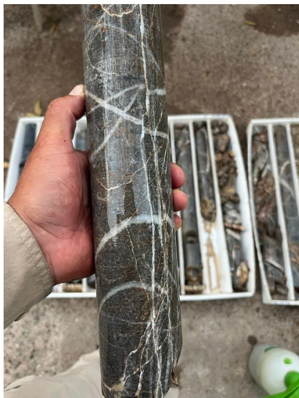
Figure 8 (left image): IE-001-2025 drill core from 177 to 180 metres showing potassic alteration and stockwork. Visually estimated grade 0.1 - 0.4% Cu. Laboratory assay results are due to be received in September 2025.
