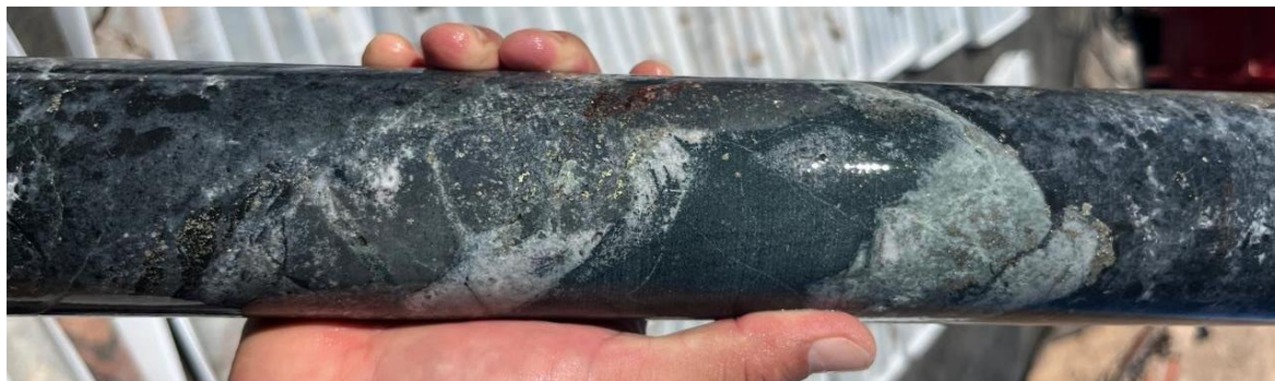
Figure 3: CAP-001-2025 drill core from 184.20 to 184.75 metres displaying tourmaline/specularite breccia with chalcopyrite mineralisation hosted in diorite intrusive. Visually estimated grade 0.5% Cu 1,16
