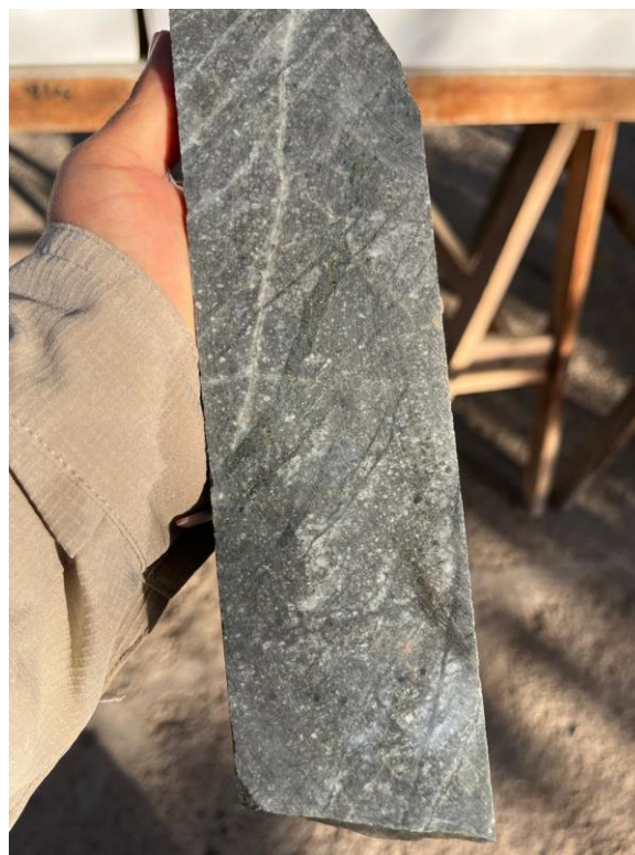
Figure 8 (left image): IE-001-2025 drill core from 177 to 180 metres showing potassic alteration and stockwork. Visually estimated grade 0.1 - 0.4% Cu. Laboratory assay results are due to be received in September 2025.
