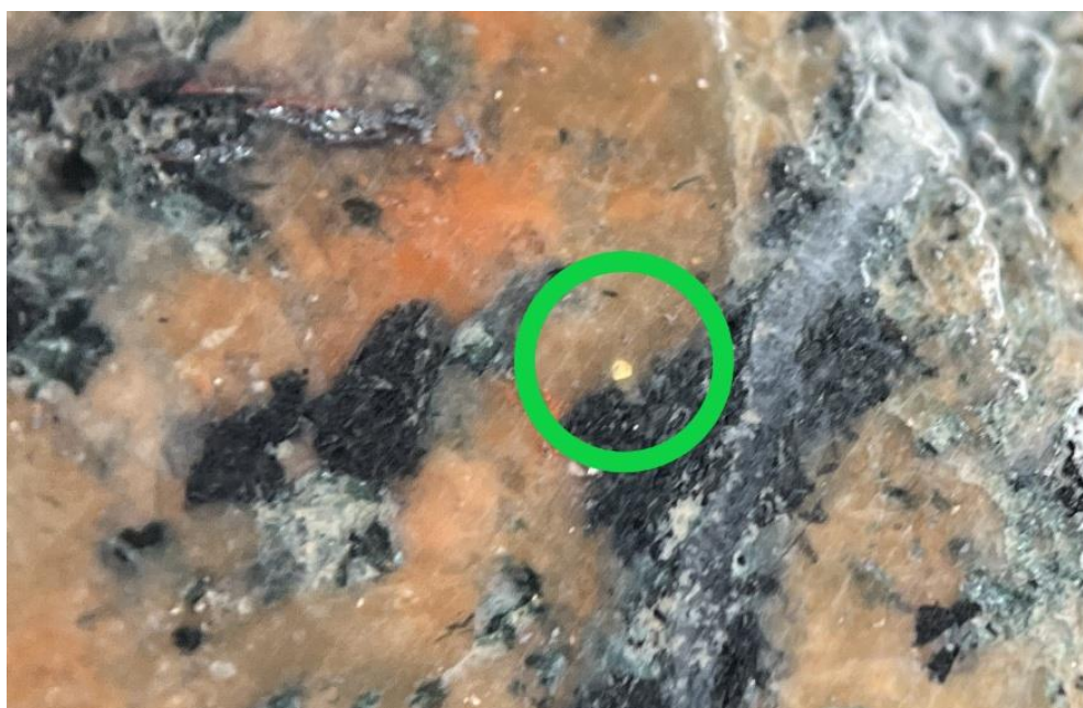
Figure 3: CAP-001-2025 drill core from 184.20 to 184.75 metres displaying tourmaline/specularite breccia with chalcopyrite mineralisation hosted in diorite intrusive. Visually estimated grade 0.5% Cu 1,16
