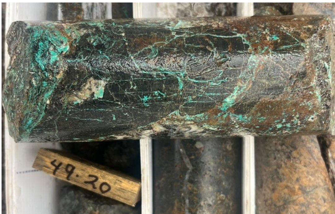
Figure 5: CAP-002-2025 drill core at 49.20 metres displaying tourmaline/specularite breccia with malachite (copper oxide) mineralisation hosted in diorite intrusive. Visually estimated grade 0.5% Cu 8
