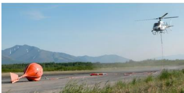
Image 1: MobileMT™ system used in Kuniko's airborne survey.
