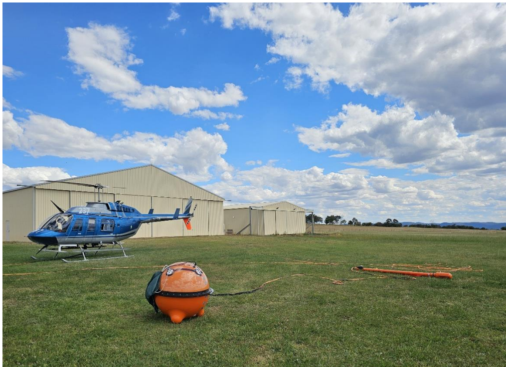
Image 3: Helicopter and MobileMT™ “bird” in pre-flight setup at the Commonwealth Gold-Silver Project, NSW.
