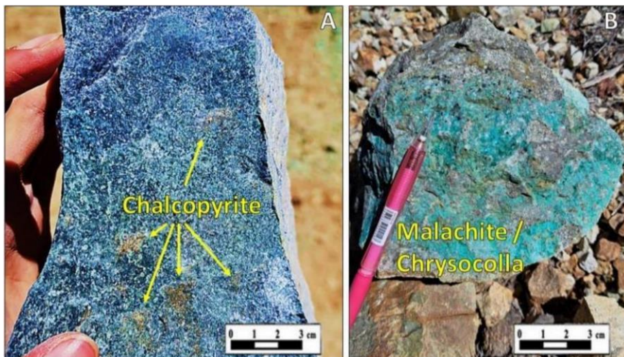
Figure 1: Example of mineralisation identified at the La Florida Prospect, A: Copper sulphide present as chalcopyrite Sample # CPO0008692 - 3.18% Cu and 2.61g/t Au, B: Copper oxide present as malachite and chrysocolla Sample #CPO0008688 - 3.96% Cu and 1.17g/t Au.
