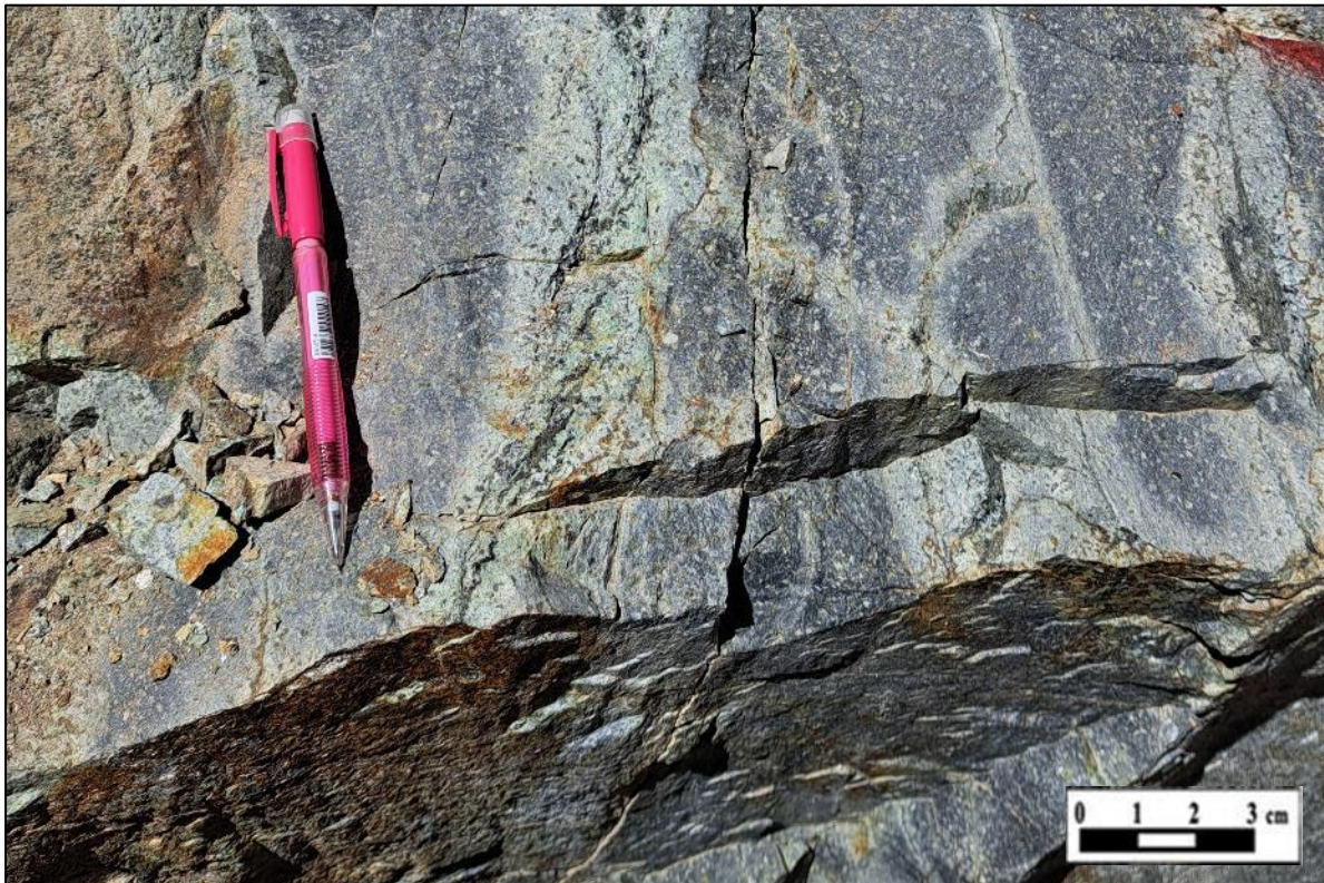
Figure 3: Strong zones of Porphyry style D-veins identified at La Florida.
