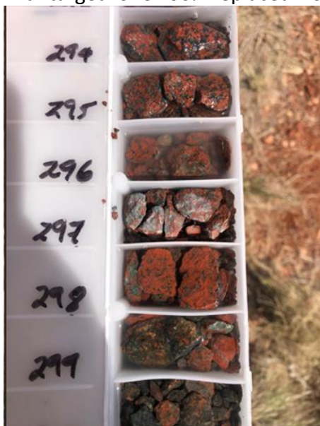
Photo 2: Example of intense redrock alteration, MFRC001
