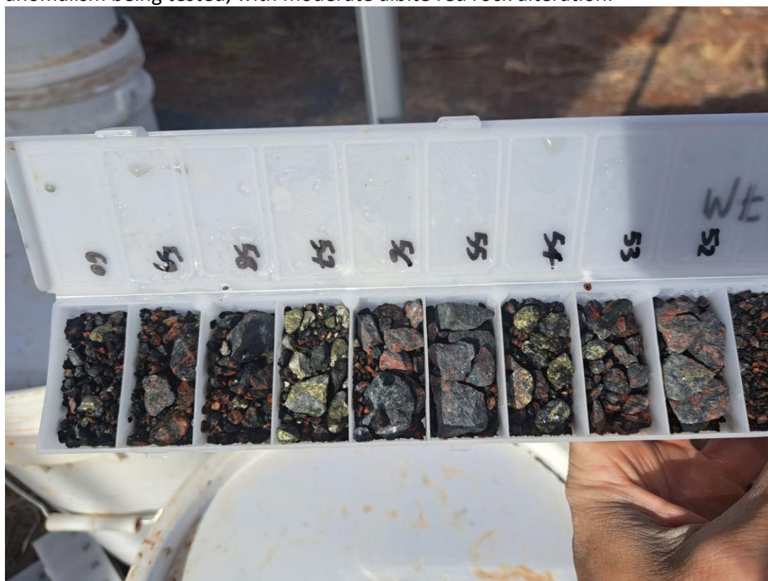
Photo 1: Chalcopyrite-rich RC chips from mineralized zone, MFRC008
