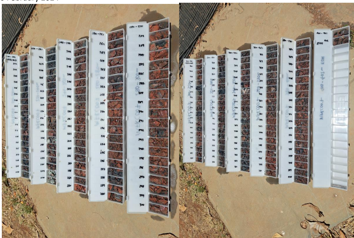
Photo 6,7: 'Red rock' alteration in chip trays, 200-402m- MFRC007.
