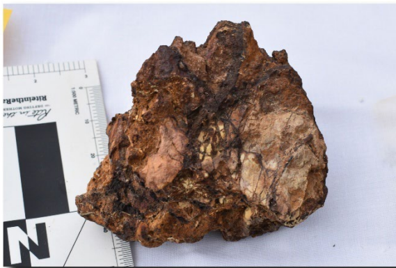
Breccia and cross-cutting veinlets, NP074. 0.007g/t Au, 1.07ppm Ag, 2,070ppm As, 214ppm Cu, 49ppm Sb, and 6,350ppm Zn.
