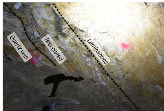
10.15g/t Au (channel sample, NP076). Laminar quartz veining with some brecciation.
