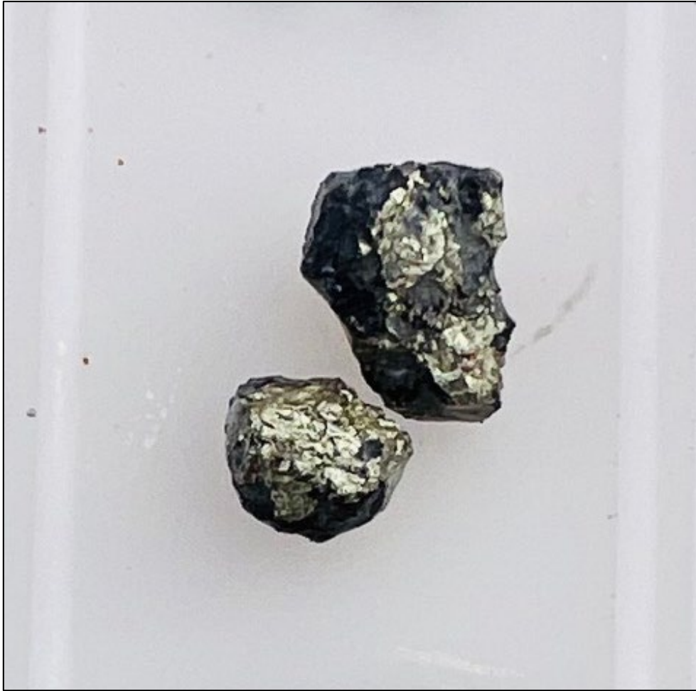
Photo 4. Close up of covellite-coated (dark blue / black) chalcopyrite (yellow) chips – the larger is approximately 5mm long.
