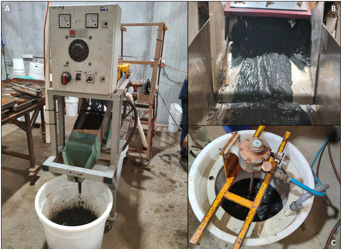
Figure 1; Photos showing A) Samples being prepared for filtration after DTR testwork completed, B) Eirez Davis Tube tester setup for sighter DTR testing and C) Magnetic concentrate produced after filtration.
