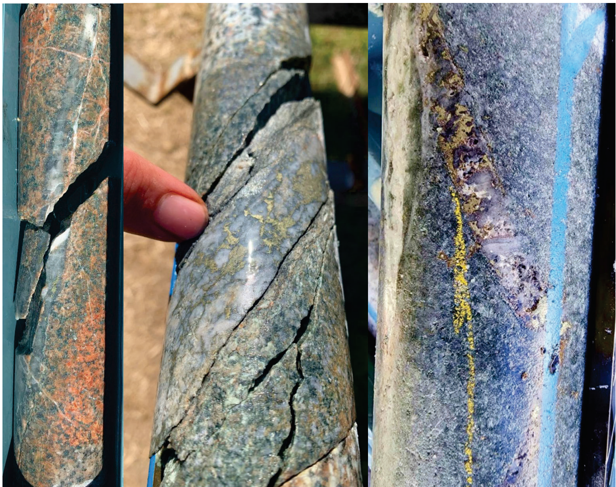
Figure 6. Left to Right. MRDD001, 227.3m strong potassic alteration of granodiorite with sulphide bearing quartz-vein (0.6m @ 10ppb Au, 0.5g/t Ag & 857ppm Cu). MRDD002, 136.15m quartz-sulphide vein within shear of strong sericite alteration of granodiorite (0.5m @ 9.35g/t Au, 21.1g/t Ag & 0.7% Cu). MRDD003, 34.9m strong silica and sericite alteration in granodiorite, quartz veins with visible chalcopryrite (0.6m @ 0.3g/t Au, 37g/t Ag & 1.6% Cu).
