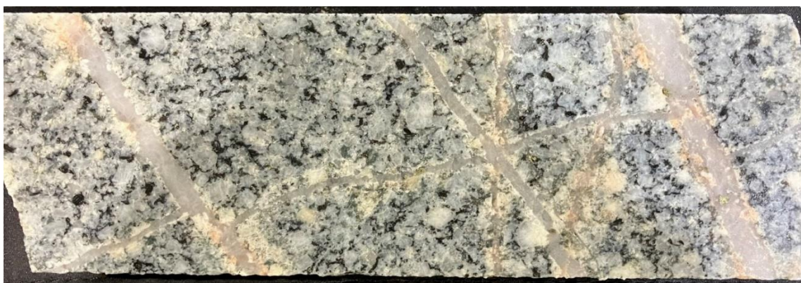
Figure 3 Mineralised and altered porphyritic granodiorite at 76.5m down-hole depth in 23BRD0016, within a 2m sample which assayed 0.31% Cu
