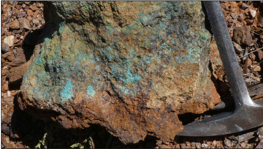
Figure 7. Sample NT0104 shows malachite staining on fractures within gossanous material, assayed 6.62% Cu, 0.10 g/t Au and 8 g/t Ag.
