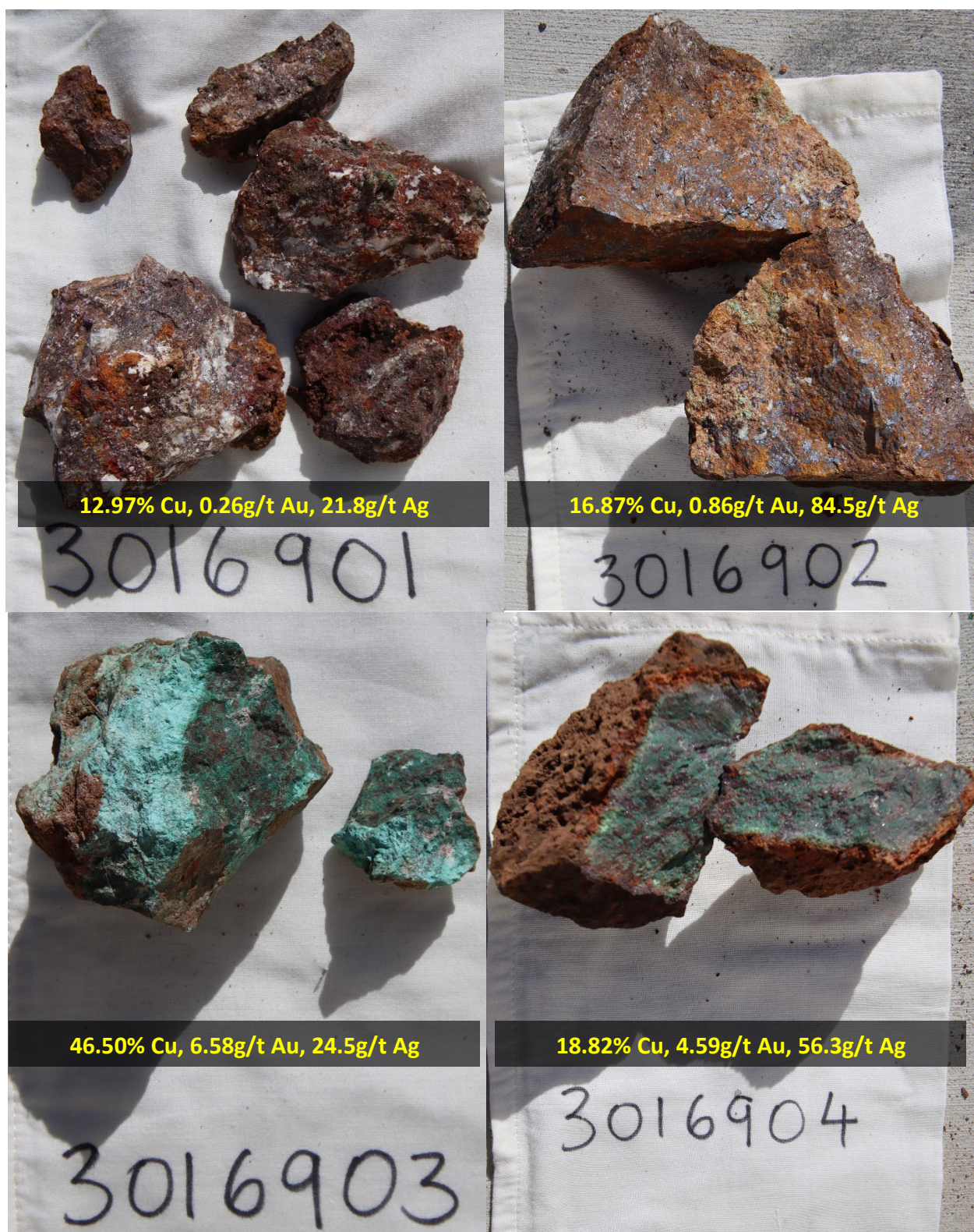
Figure 5. Recent mullock and rock chip samples collected from the Halls Reward Prospect. Descriptions are as follows: Sample 3016901 – copper oxide bearing ferruginous quartz, altered rock, iron oxide, native copper and malachite; Sample 3016902 – copper oxide bearing ferruginous quartz, altered rock, iron oxide, native copper, cuprite and malachite; Sample 3016903 – copper oxide bearing chrysocolla, malachite, ferruginous clay quartz and altered rock; and sample 3016904 – copper oxide bearing ferruginous siliceous gossan, iron oxide, malachite needles, cuprite, spongy silica, clay and altered rock. (Refer to ASX announcement dated 10 September 2025)
