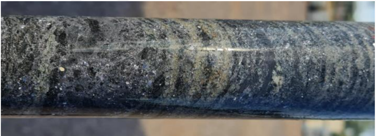
[Figure 1] Strongly galena mineralised zone with carbonate gangue from the Shallow Silver Zone along the Eastern Horizon.
