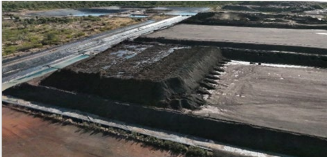
Figure 2. Mt Norma mine: Approximately 50kt of copper ore oxide undergoing leaching
