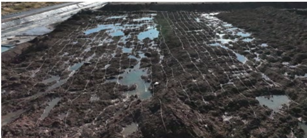
Figure 4. Mt Norma Mine: Stockpiled copper ore oxide undergoing leaching
