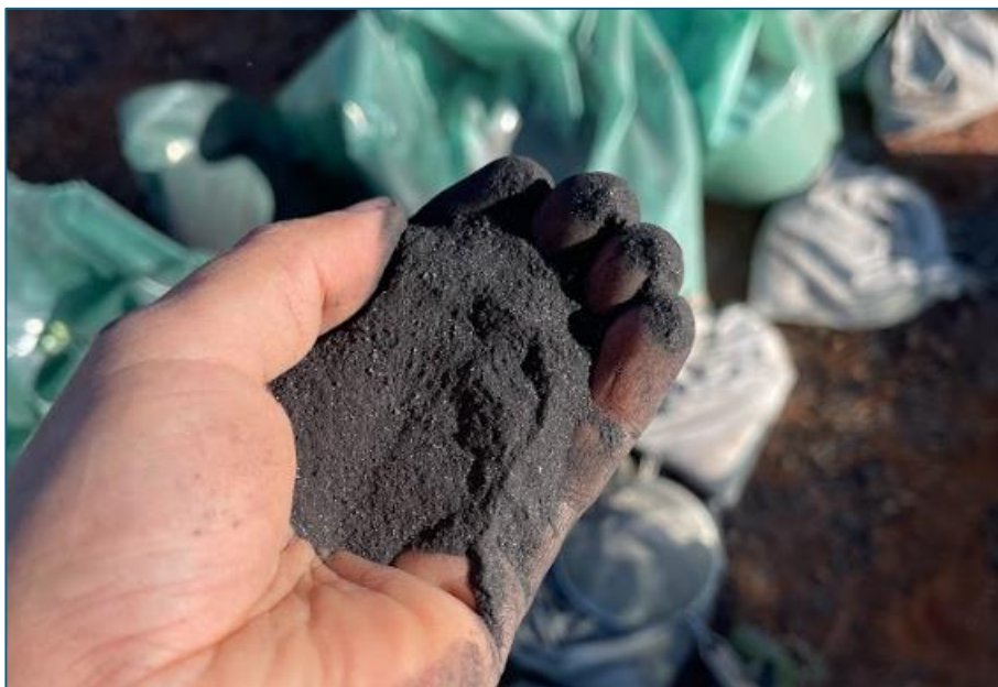
Figure 2: Typical black-coloured, heavy magmatic sulphide mineralisation at the Dante Reefs (HRC004).
