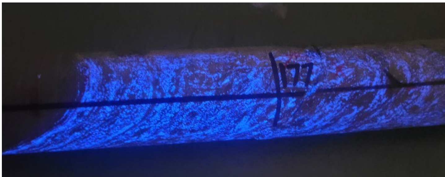
Figure 2 – WQDD013 (0.65m @ 18.35 WO 3 ) scheelite intersection under UV light
