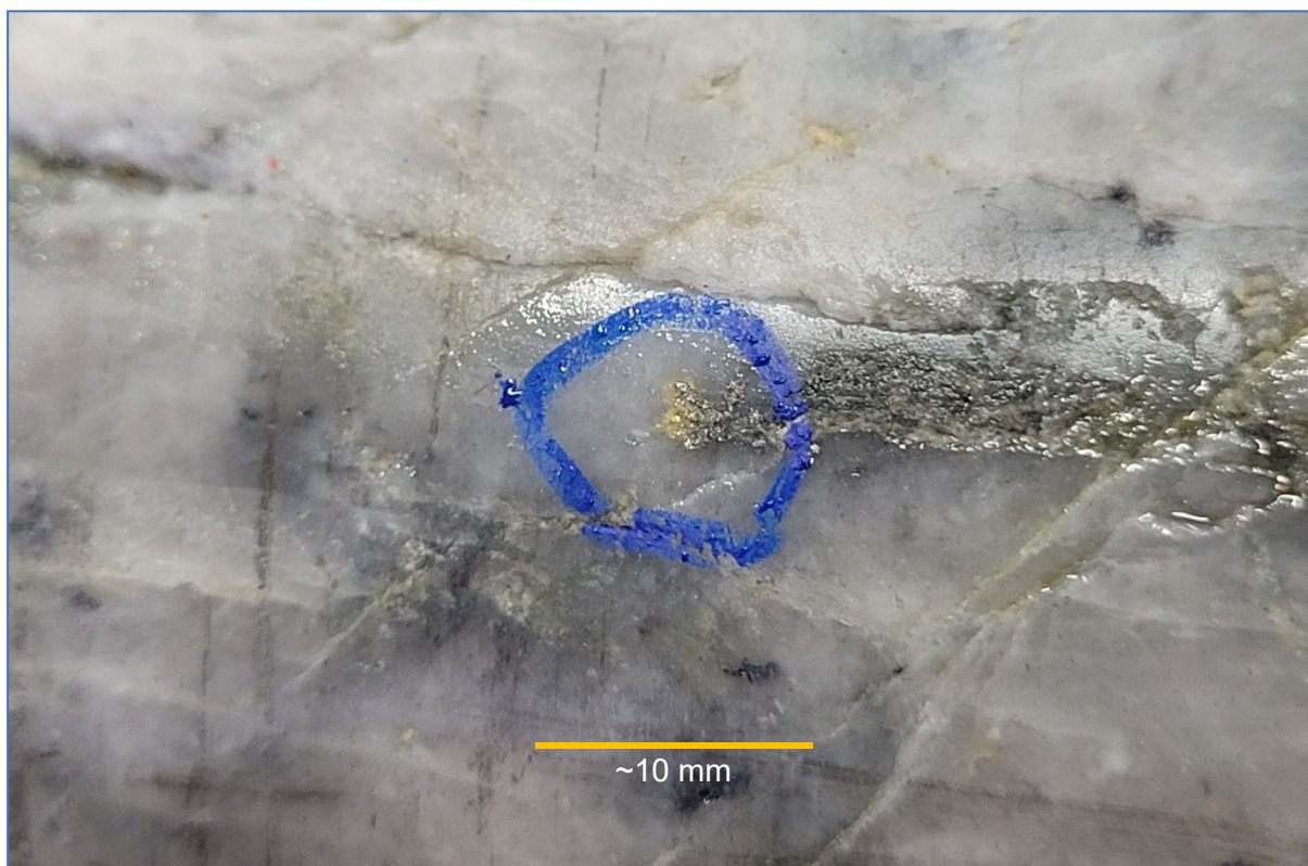
Figure 5 - TFDD013 drill core - visible gold (circled) at ~26m depth
