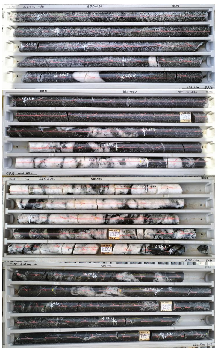
Figure (4): Achilles Diamond Drill Hole MDD026 –Granodiorite/basalt western contact zone 422.1m – 438.4m down-hole.
