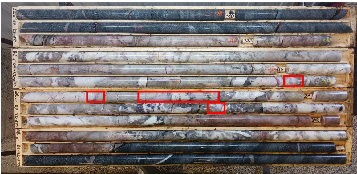
Photo 2: Core from Hole CLO-063 exhibiting crystalline pollucite (internal to the pegmatite dyke) over 3m, between 337 m and 340 m, of approximately 3-8% pollucite (visual estimate, red outline), and 10m from 334 m - 344m visual estimate of crystalline spodumene (internal to the pegmatite dyke) is between 5% and 20%. 2
