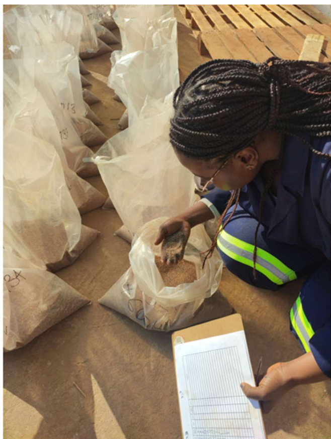
Figures 5 & 6: LHS: Inspection and logging of oversized material & RHS: Rutile-rich HMC prior to despatch for dry separation
