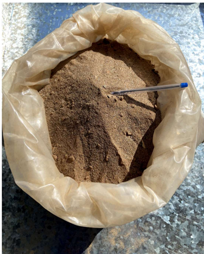
Figures 5 & 6: LHS: Inspection and logging of oversized material & RHS: Rutile-rich HMC prior to despatch for dry separation
