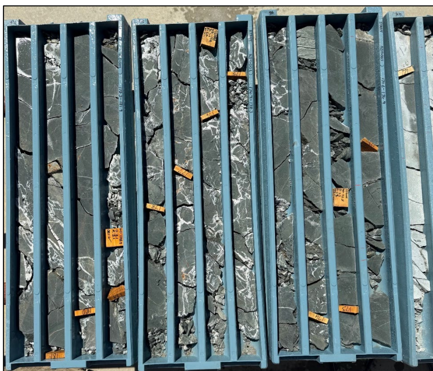
Photos 4. Core tray photos showing brecciated and quartz-carbonate matrix interval from 173.4m to 192m down hole in SJD001 (1½ cut HQ3 drill core).
