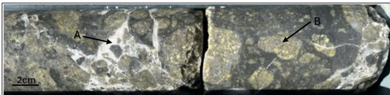
Figure 4: Breccia comprising calcite matrix (A), with clasts of rhyolite (B), black silica and black shale from Main Vein in 25FCDD014.
