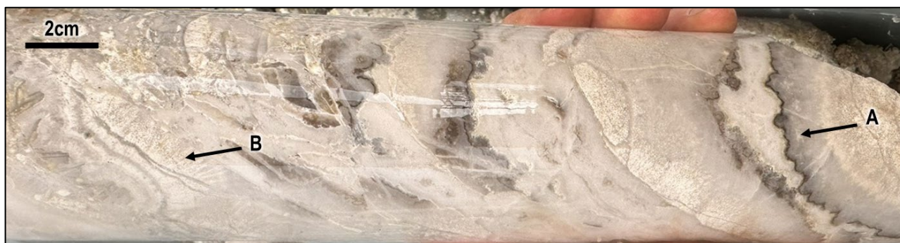
Figure 1: Marcasite colloform (<1% vein fill, A) within colloform – crustiform, quartz – adularia (B) from from high-grade A-Vein interval reporting 1.4m @ 31.70g/t Au from 55.8m depth in 25FCDD007.
