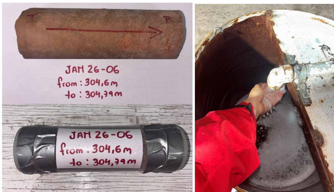
Figure 1. Core extracted at 304.6m ready for porosity testing and brine flowing in packer test ready for assay.
