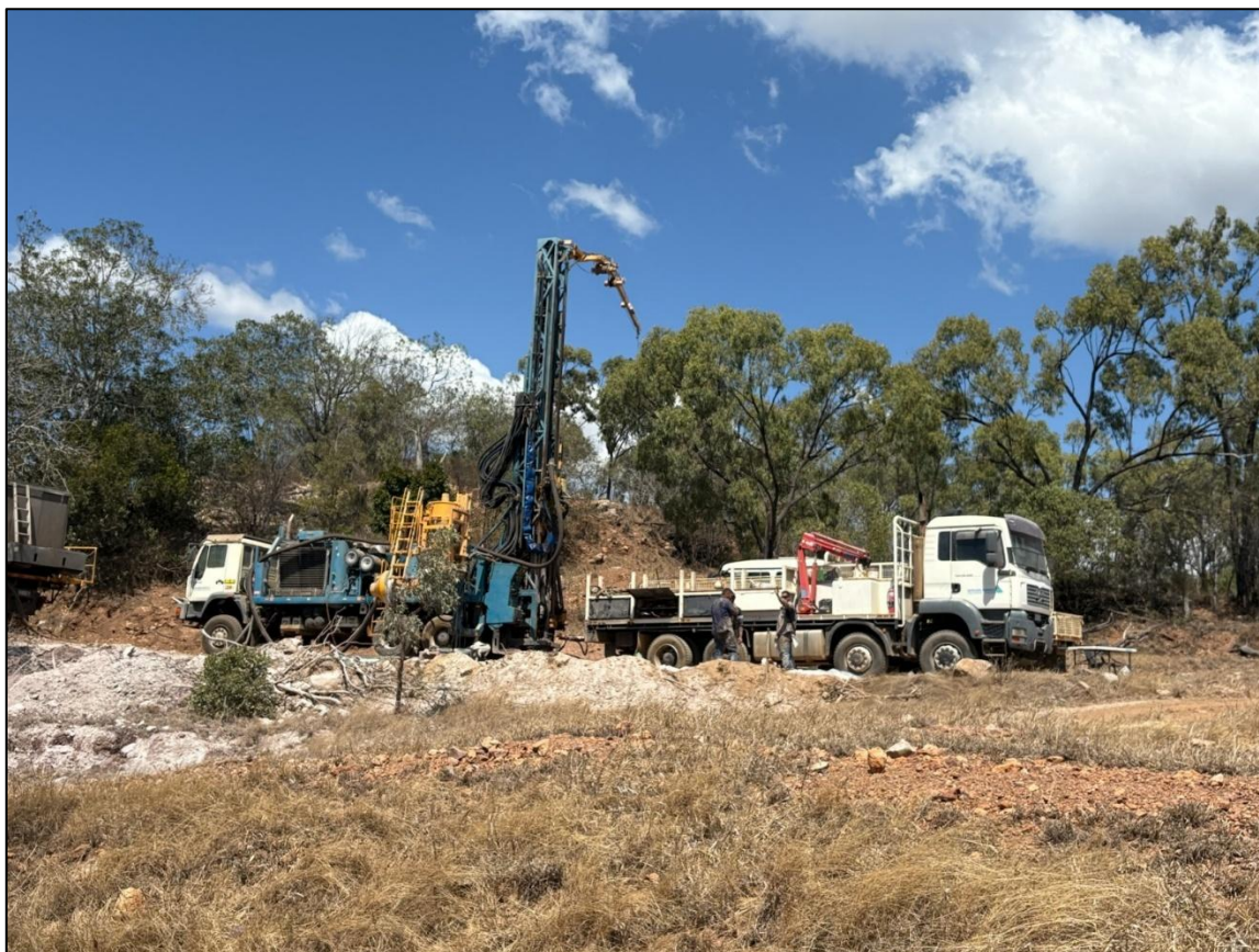
Figure 1: RC drill rig completing maiden drill hole at Mount Mackenzie.
