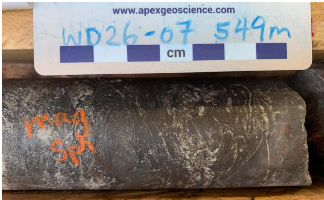
Figure 4: Semi-massive visual sphalerite (brown) in NQ drill core from approximately 549.0m downhole in drill hole WD26-07. Laboratory assays for this interval are pending.
