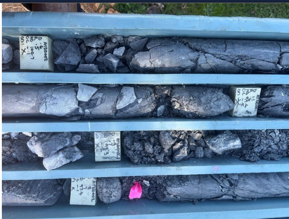
Figure 5. Drill core from ATDD002 for the drill run of 93.8m to 100.7m down hole showing the mineralised vein in context (pink arrow). Core diameter 47.6mm.
