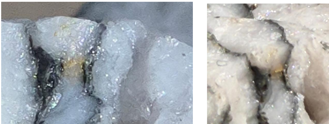
Figure 2. Visible gold 1 grains (lustrous yellow) up to 1mm and sulphide minerals in quartz veining in hole ATDD002 at 91.8m down hole. Core diameter 47.6mm. Assays are pending for this hole
