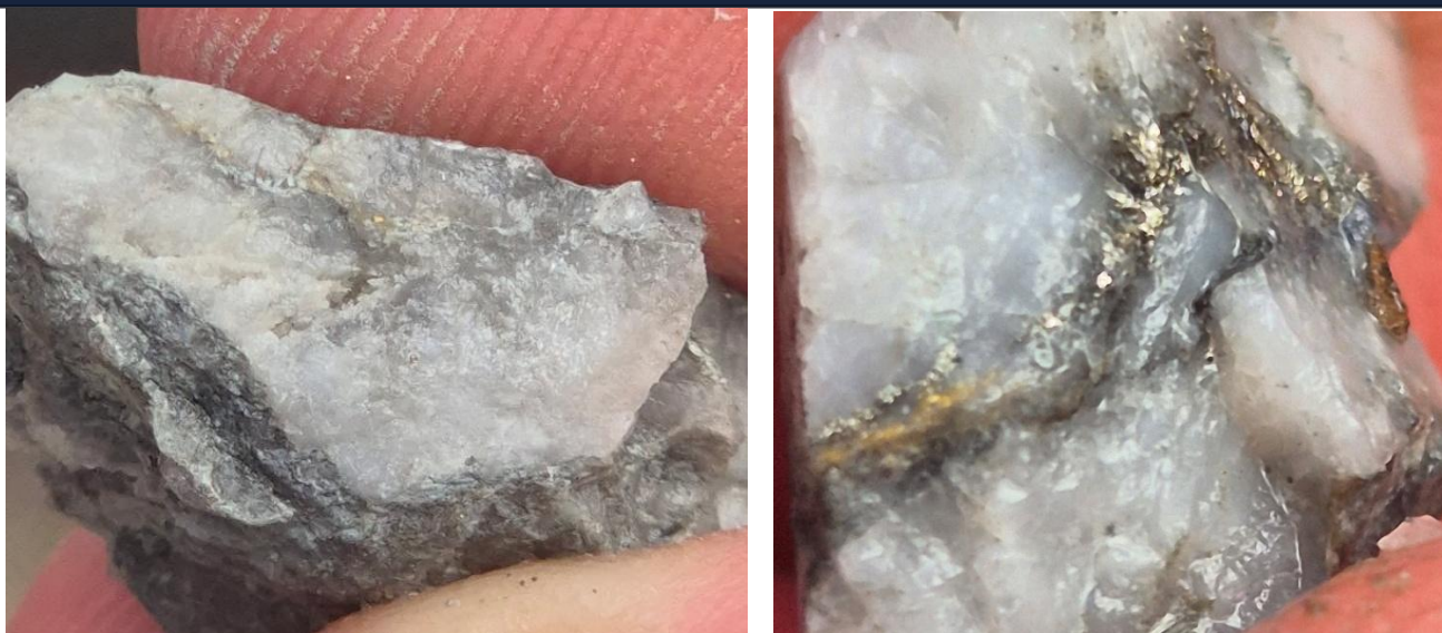
Figure 3. Visible gold 1 grains (lustrous yellow) up to 2mm and sulphide minerals, in quartz veining in hole ATDD002 at 98.1m down hole. Core diameter 47.6mm. Assays are pending for this hole.
