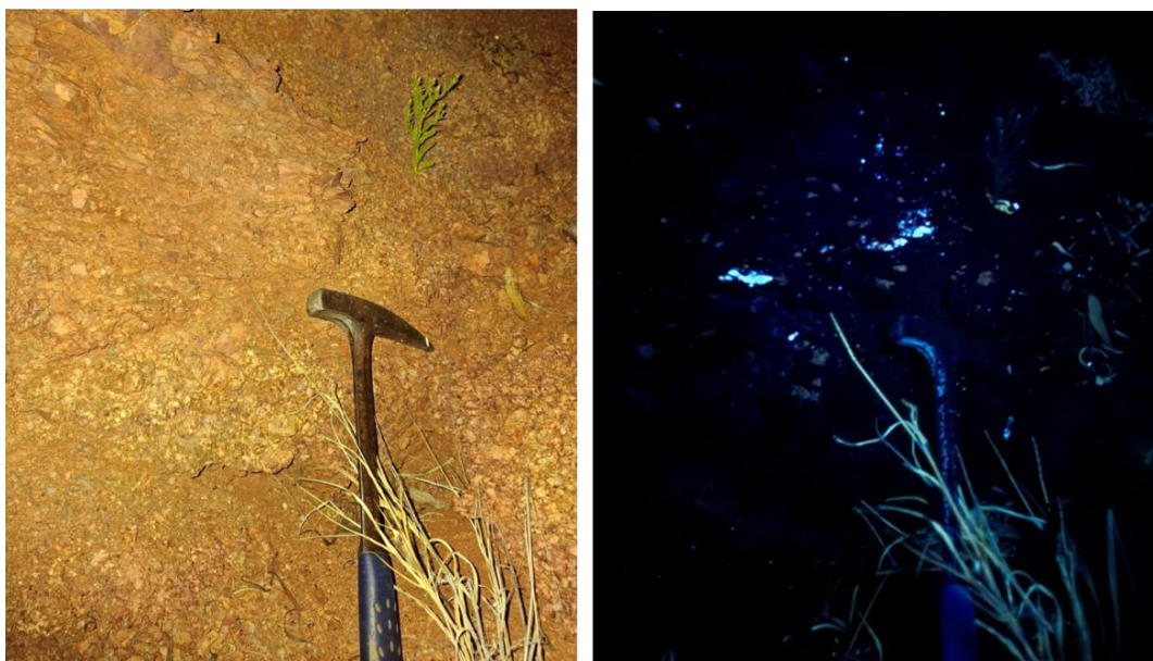
Figure 2: UV (right) and white light (left) lamping photographs showing UV fluorescent mineral response (estimated at ~5% scheelite) in porphyritic granite at Hill of Leaders Project NT.
