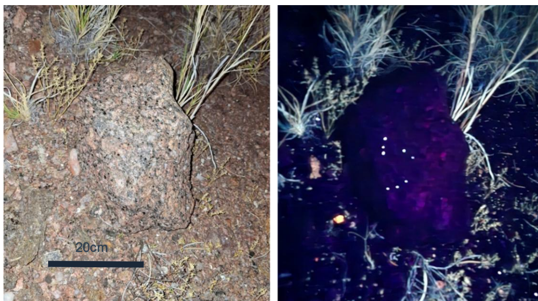
Figure 1: UV (right) and white light (left) lamping photographs showing UV fluorescent mineral response (estimated at < 1% scheelite) in porphyritic granite boulder at Hill of Leaders Project NT.
