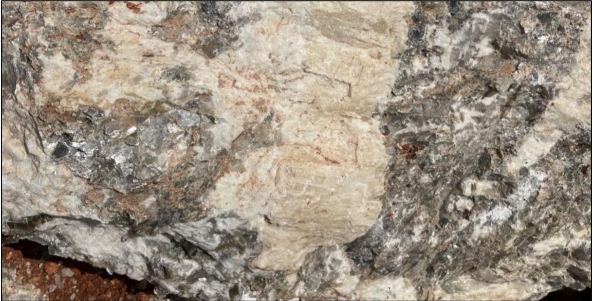
Figure 5: Pippingarra Project Hand specimen showing flake mica (grey), with potassium feldspar (cream), albite (white) and quartz (grey).
