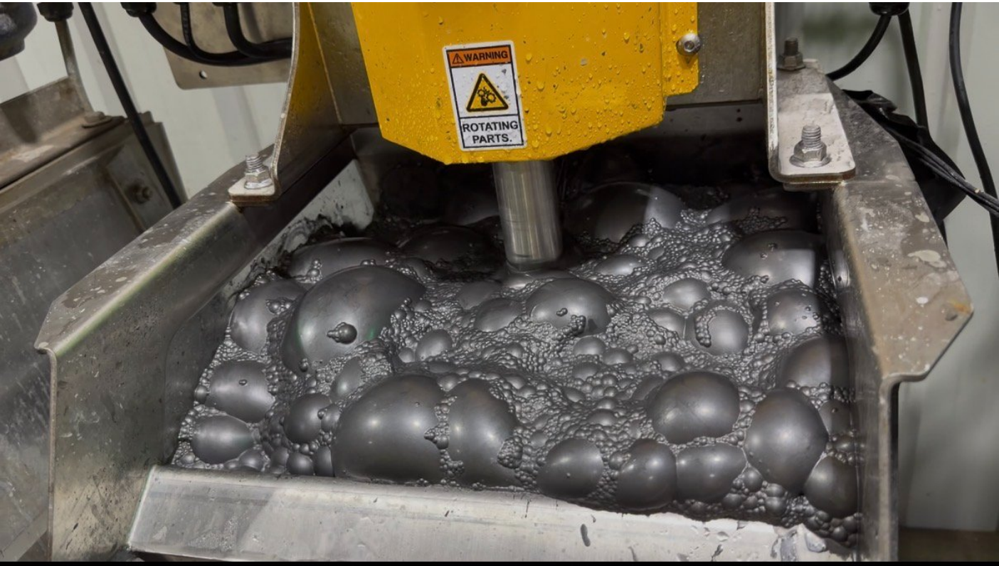
FIGURE 4 — SULPHIDE FLOTATION, REMOVAL OF GANGUE SULPHIDE MATERIAL
