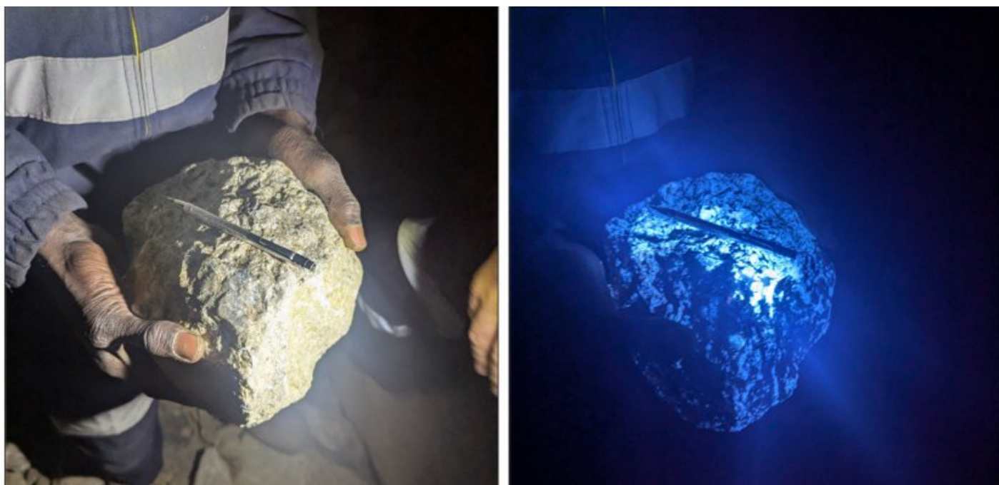
FIGURE 8 — ROCK CHIP FROM THE BULK SAMPLE ZONE, 16.9 KG GRADING 64.3% WO 3 , UNDER UV LIGHT
